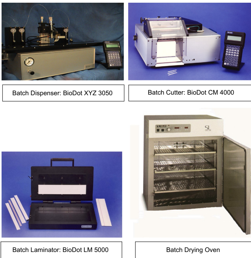
FIGURE 3 Typical batch manufacturing equipment. (The color version of this figure may be viewed at www.immunoassayhandbook.com ).
